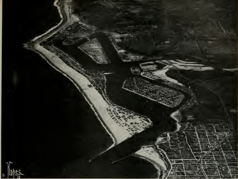
Air view of Newport Harbor. Note the Beach on the Ocean Front. The difference in color about half way of the width of the beach indicates where the fill from the Bay dredging begins. The outer half of the beach is nearly all filled in area. (Courtesy Kopeck Photo Co.)
